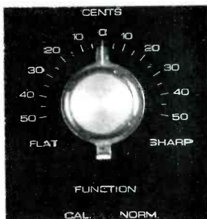
Fig. 7 The CENTS knob and separate pointer has a double function. It's used first for calibration, then the pointer is turned to zero, allowing a variation of half a semi-tone flat to a half semi-tone sharp from correct tuning. Combined with the SELECTOR, this gives continuous coverage.
