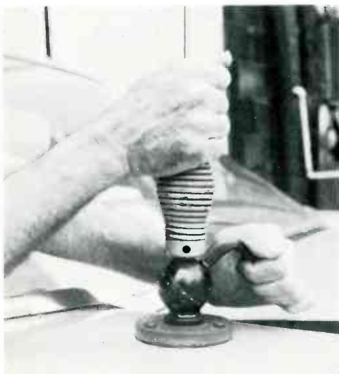
Fig. 6-12 Method of positioning the mobile whip.
