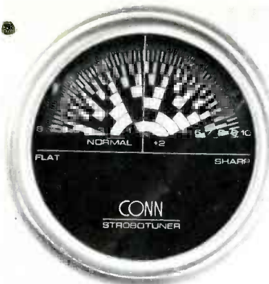
Fig. 3 There are eight semi-circular bands of lines visible through the window. Each band is a different octave. The normal octaves are marked on the left, the +2 octaves (octaves 2 through 10) are labeled on the right. With correct tuning, the lines of one or more bands appear to be motionless. When the note is flat, the lines move to the left (counterclockwise), or sharp notes move the lines to the right (clockwise).
