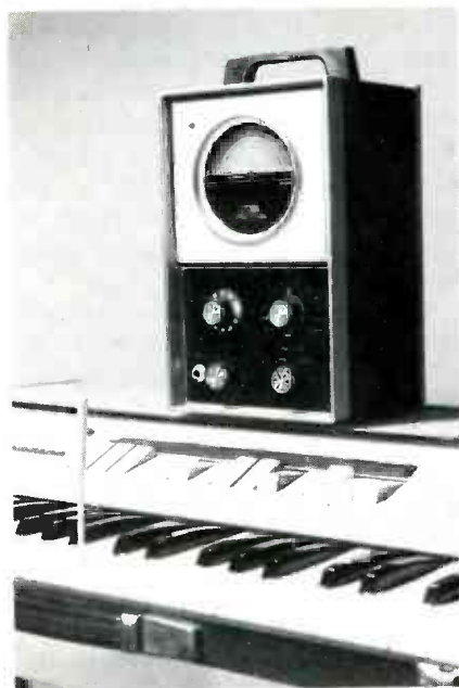
Fig. 2 The Model ST-11 Strobotuner is ready to be connected to the organ that needs tuning.
