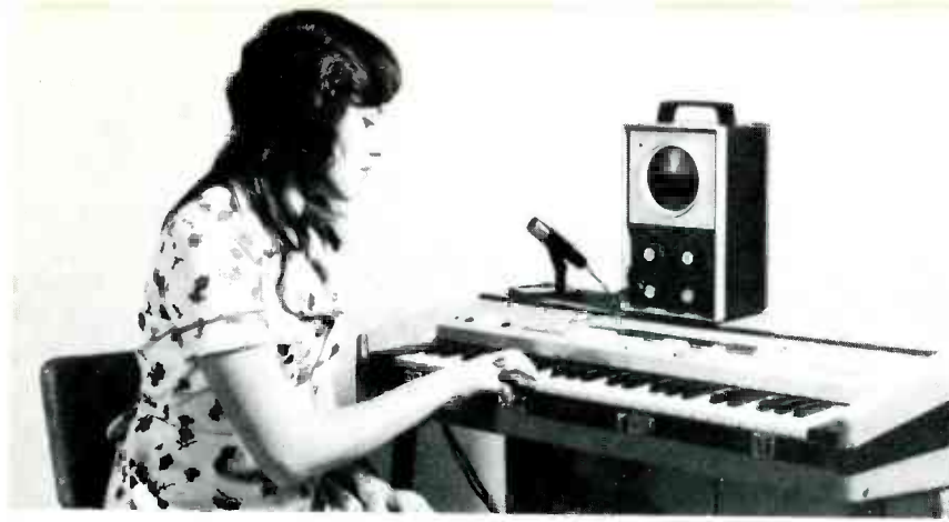
Testing or resetting the tuning of an electronic organ is easy and fast, with the Strobotuner.
