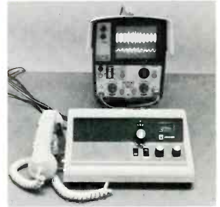
Fig. 12 With a Tektronix Model T932 scope, one channel can be connected direct to the 27-MHz modulated RF output signal (top trace), while the other channel shows the audio recovered by another radio.
