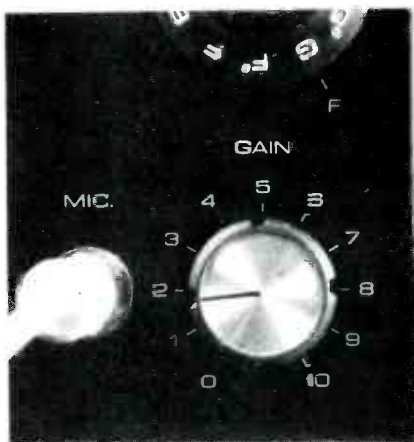
Fig. 5 At the lower left corner of the panel are the microphone jack and the GAIN control.
