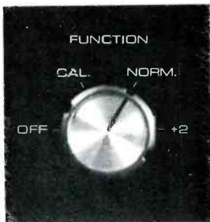
Fig. 6 In addition to controlling power on/off, the FUNCTION knob selects calibration, the normal tuning function, or the special +2 tuning circuit which increases the top range by two octaves.
